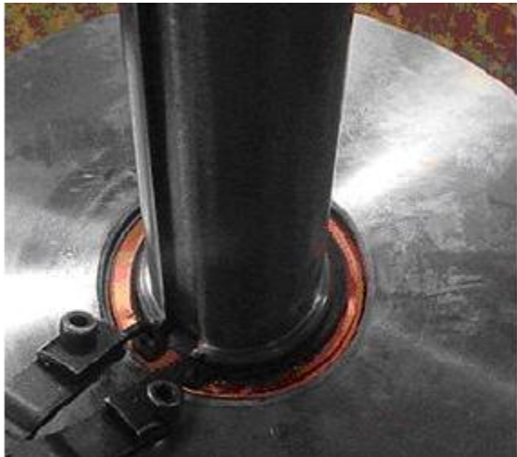
Remove snap ring and take off stationary driven varidisc to see brake shoe
