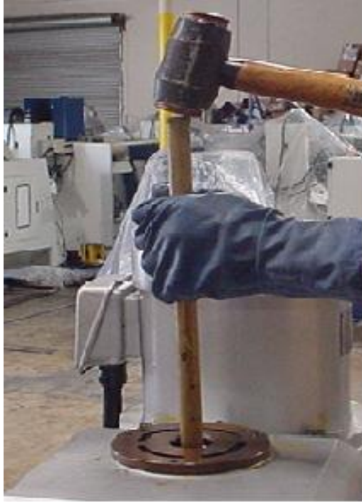
One person hold spindle R-8. Another one use brass bar and hammer to hit spindle down.
