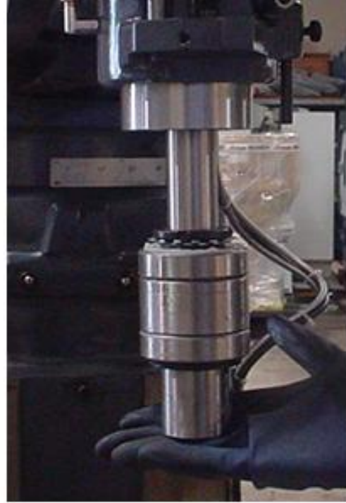
One person hold spindle R-8. Another one use brass bar and hammer to hit spindle down.
