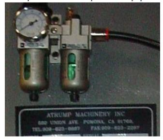
2. Install air regulator unit at the left side on the top of the tag.
