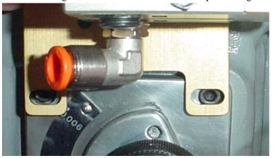
3. Install the control bracket. Remove two screws and replace with longer screws (provided.)
