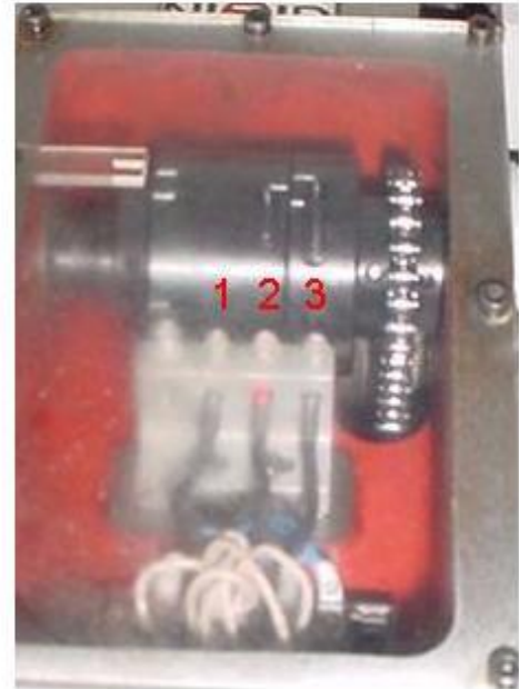
1 : Arm At Home Input Sensor. 2 : Arm At Clamp Input Sensor. 3 : Arm At Stop Input Sensor.
