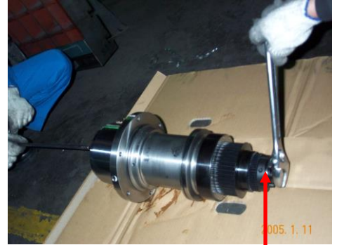
Hold the end of the spindle with a wrench
