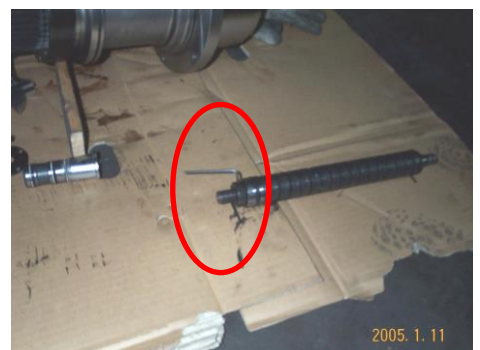
Loosen 2 M5 headless screws and remove the lock
