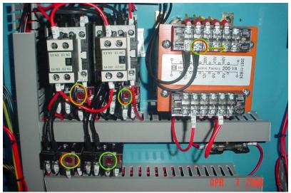
2. Change wires input to Spindle motor from 220v to 440v.
