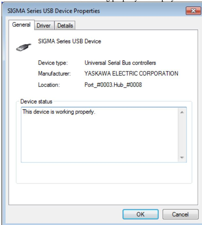
When "This device is working properly." is displayed, the SERVOPACK is ready to be used through a USB connection. If it is not displayed, reinstall the USB driver.
