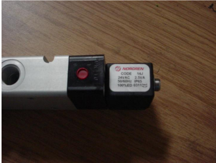
Picture 1. 24V Voltage Mist Solenoid Valve.
