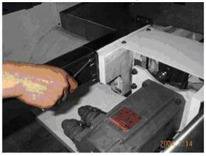
(3) Than use dial test indicator for checking after fitting support, support must be lower than the slide way surface 0.03~0.05mm; Checking the side face of support by dial test indicator, the base of dial lean on side of slide way to check, Side face of supporter must be lower than the slide way surface 0.01-0.15mm.
