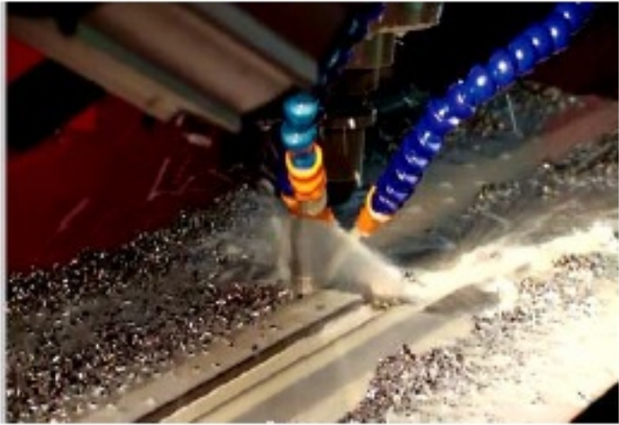
Tooling: \varnothing 18 mm 2 flute facing cutter Material: S45C , Spindle speed: 1500 rpm, Feed rate: 500 mm/min,
