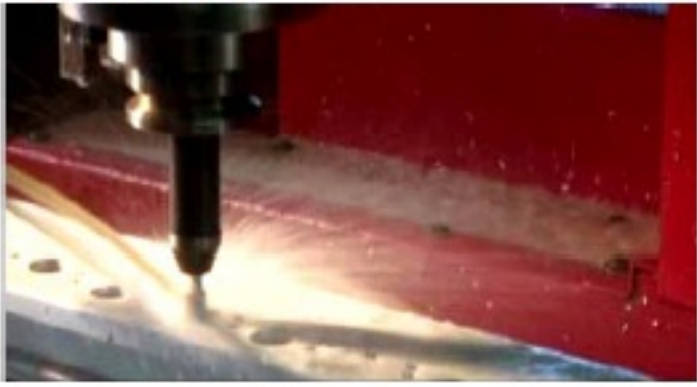
Material: Aluminum, Tooling: \varnothing 6mm end mill Spindle speed: 6000 rpm, Feedrate: 500 mm/min
