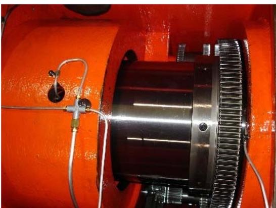
Gears in the headstock are made of chromium molybdenum steel (SCM-21), treated by cementation then precisely ground to provide smooth and quiet running. The spindle is supported by precision taper roller bearings.
