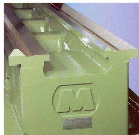
The extra-wide 450mm bed is constructed of Meehanite casting for maximum rigidity, The pre-stressed bedways are induction heat-treated and ground for wear resistance
