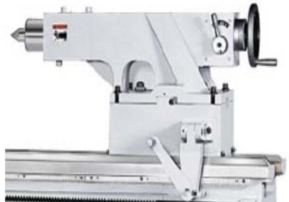
The cross slideways are hardened and ground, the saddle slideways are covered with Turcite to reduce friction. A heavy-duty casting design for maximum rigidity to support work pieces or tooling. With MT #5 taper,
